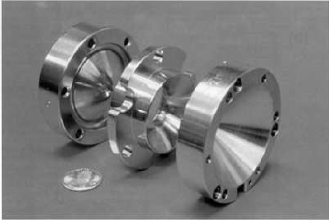
Figure 3. “The three electrodes of the quadrupole ion trap shown in open array.” [78]
